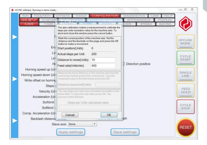
The calibration is built from a 3 steps sequence. Press the OK button to process the sequences.
