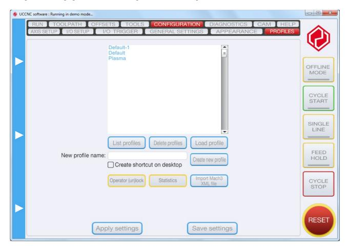
The Profile files are named as the name of the profile and has a .pro file extension. Each profile is stored in a separated file. The .pro files are plain text files with key entries, the files are therefor editable manually too with a notepad, but we recommend not to edit it this way, because a mistype can cause the key to be unreadable for the software.
