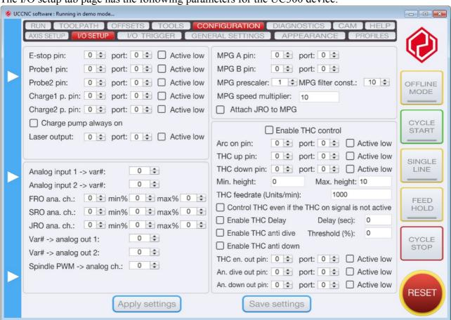
**E-stop port & pin:** This is a physical input pin for the e-stop button input signal. The pin can be inverted checking the active low checkbox next to the textfield. The machine goes to reset when this input signal is active.
