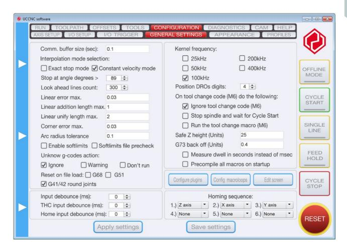
**Exact stop mode:** This is a trajectory planning mode. In this mode the trajectory planner follows the motion path positions exactly. The machine axis accelerates at the beginning of each segment and deccelerates at the end of each segment. This interpolation mode is adviced to set if close tolerance parts are manufactured. The position error is always zero with this interpolation mode.
