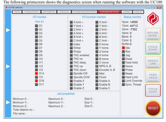
The diagnostics screen when running the software with the UC300-5LPT:
