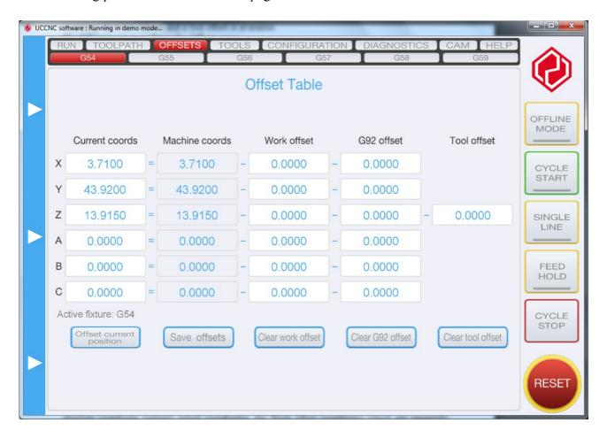
The offsets page contains 6 sub tab pages, these are the G54, G55, G56, G57, G58 and G59 offset pages respectively. These sub tab pages are identical and each of them is a different fixture. The fixtures can be selected with programming G54 to G59 in the G-code program or in the MDI.
