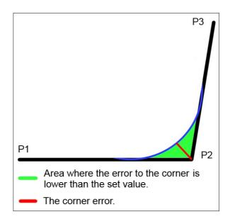
The motion path is calculated in a way that the new faster path contains the error at these connection points lower than the set value. In the following graph an example connection and new path calculation is demonstrated. The green area is where the corner can be rounded. The machine can move anywhere in the green marked area and the fastest possible path will be selected by the motion planner. The parameter is in Units.
