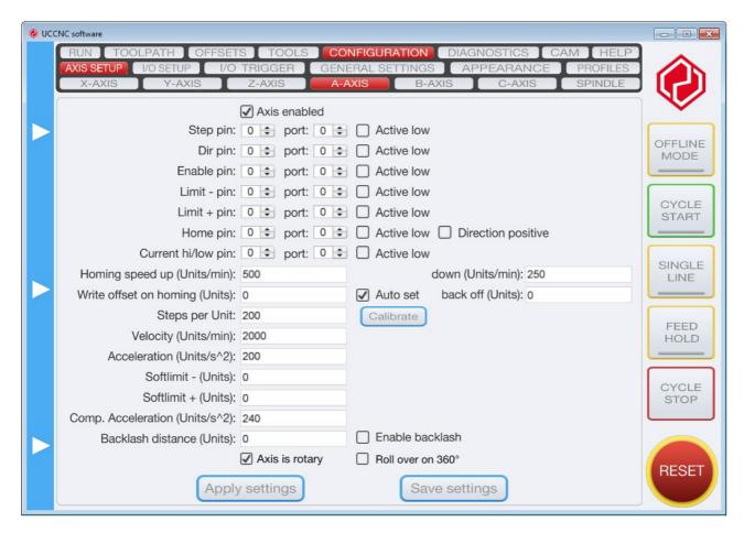
The A axis can also work as a tangential cutter knife when the A axis rotation angle is automatically calculated and rotated to the XY plane movement vector direction. This way a motorised rotary knife can be used to cut foil or sticker sheets for example.
