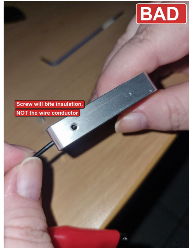
BAD — grub screw will bite into the black insulation, NOT the wire conductor
