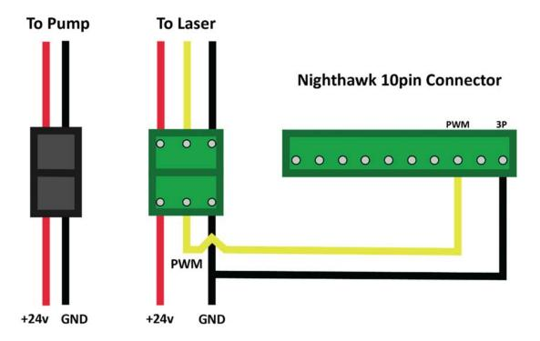
If you have already had a laser set up and running from your Nighthawk, or you have one of our pre-built machines you will need to remove the Red Yellow and White cables from the long 10-pin connector on your controller and instead they will need to be inserted into the green 3-pin connector that came with your kit but be careful to match the colours of the wires!
