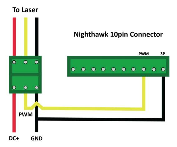
In this example, the DC+ and GND wires are coming from the power supply and are powering the laser. The yellow PWM wire on the supply side is coming from the PWM pin on the Nighthawk however it needs a return path which is the black wire in the 3P pin. This 3P wire needs to connect to the GND wire. It doesn't matter which side of the 3-Pin connector it goes to but we have found it easier on the supply side rather than the laser side.
