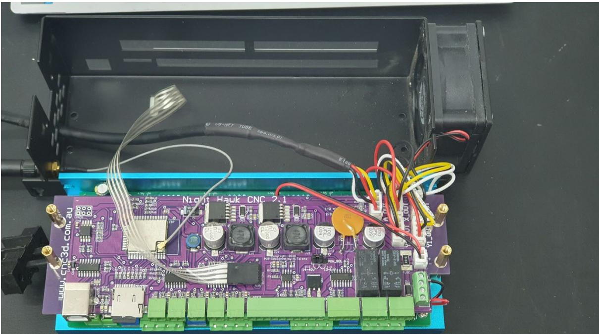
Step 8: Reverse steps 1-5 to close the case. Pay close attention to the red and black fan cable and the coloured motor cables as they can easily get pinched in the case.
