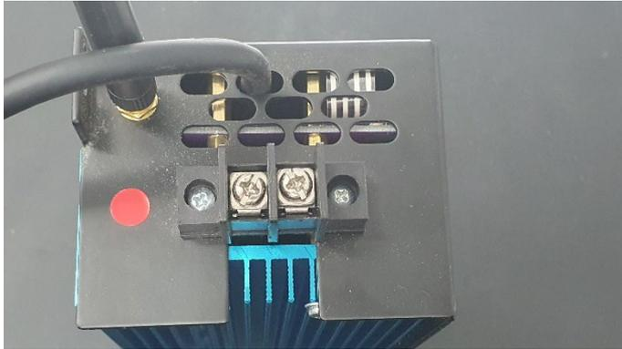
CNC3D's 4-Core stepper cable fits through the grid holes on the power supply end of the Nighthawk.
