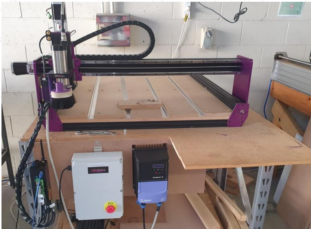
Mounting suggestion using the existing MDF electronics mounting board
