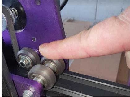
Keep in mind, with a router fitted it can put some forces on the front of the X and Z axis, this can make some wheels feel tighter than others. It's OK for the wheels to have more resistance than others in this case. You can try taking the load off the router by supporting its weight with one hand while testing the wheels with the other.
