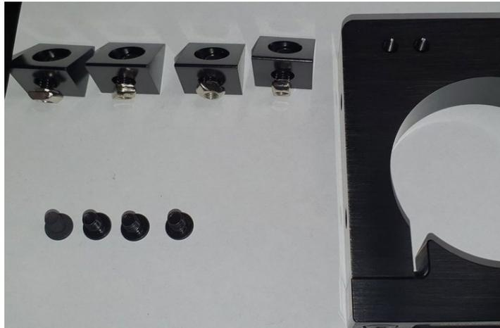
2. Loosely fasten the angle brackets towards the rear of the router in the outer edge mounting holes
