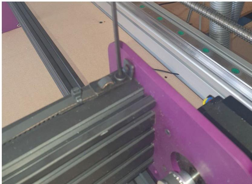
3. Now we are going to set up the bottom of the machine. You will have 2 longer 2020 extrusions and 3 shorter extrusions with a right-angle bracket on the ends. Take the 2 longer pieces and slide them onto the front and rear plates and secure the T-nuts on the plates.
