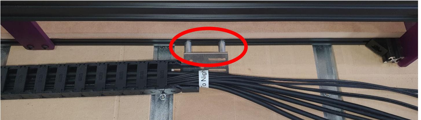
2. Remove this bolt from the left-hand side plate to allow you to secure the middle of the wiring loom to the side plate. Insert the mounting bracket and re-tighten the bolt.
