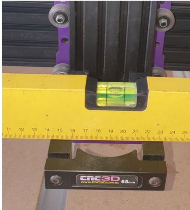
4. Loosen the front bolts on the router clamp and insert your trimmer. Ensure when fitting the router that the bottom of the collet nut sits just below the Z axis to ensure it is the lowest point. It is recommended to secure your router with the clamp as low as possible but if you are using a dust shoe make sure to leave an allowance for it.
