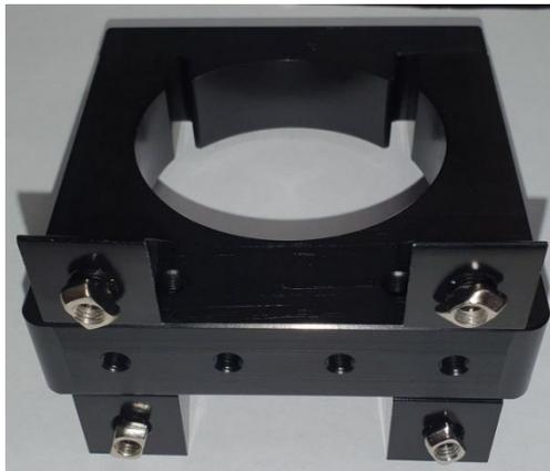
3. Attach the router clamp to the front of the Z axis loosely and use a spirit level to get the router clamp relatively level then tighten all bolts to hold the clamp to the Z axis.
