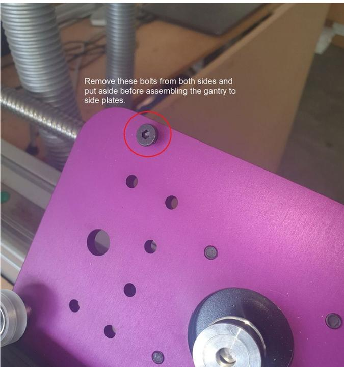
Remove these bolts from both sides and put aside before assembling the gantry to side plates.
