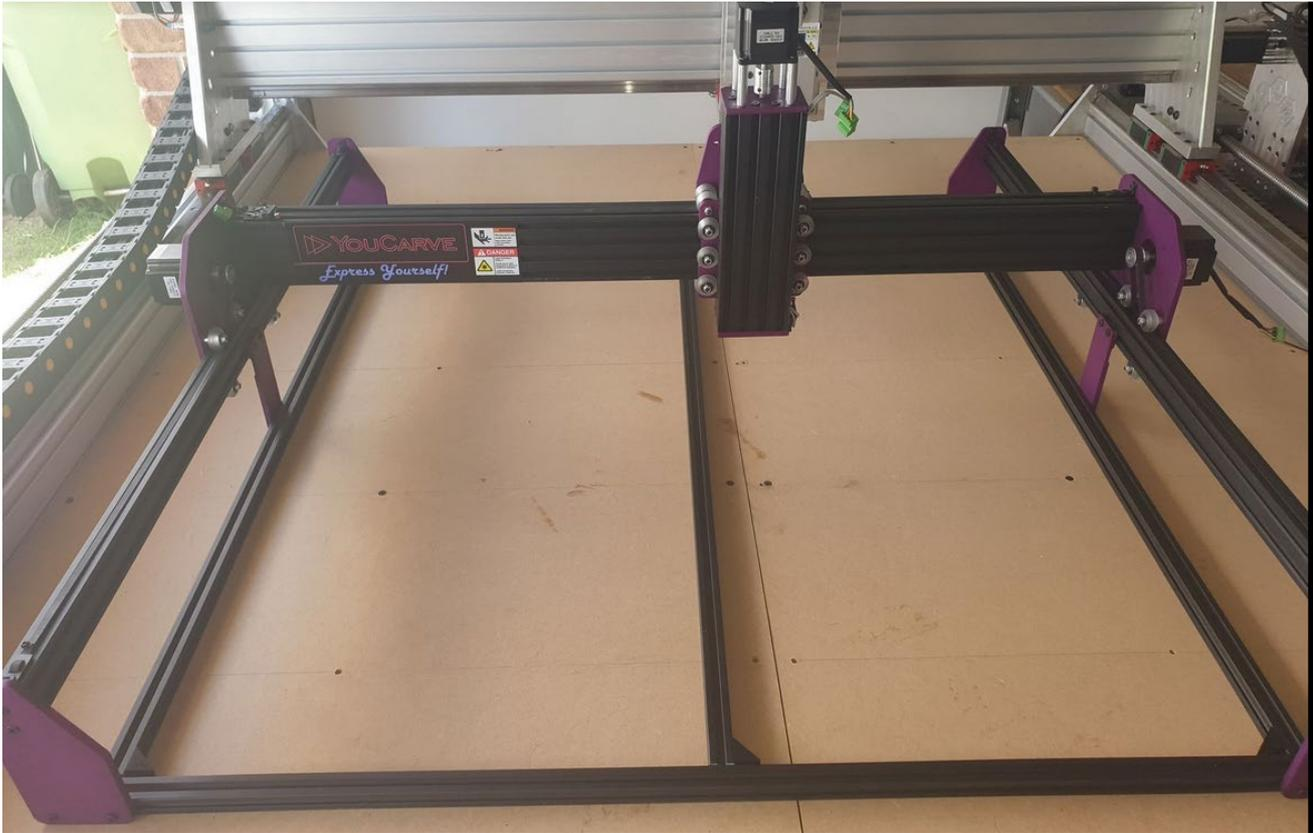
**YouCarve V2:** You will notice some 20mm spacers that have been attached to the machine frame, these have been strategically placed to contact your limit switches so they must stay attached. Please check to make sure the bolts are tight and secure.
