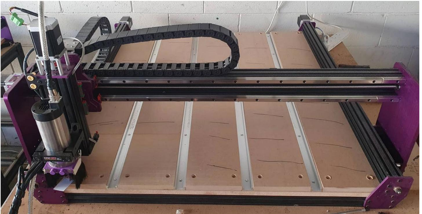
Using the jogging buttons in Commander, put a piece of scrap paper under the surfacing bit and lower the Z down until it is just touching the paper. Ensure to reduce your downward travel distance as you get closer to the surface to ensure the machine does not crash into the spoil board.
